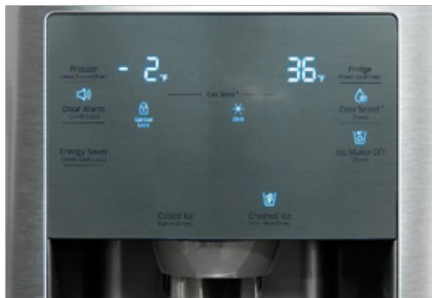
Fig. 1: Samsung Refrigerator Control Panel
