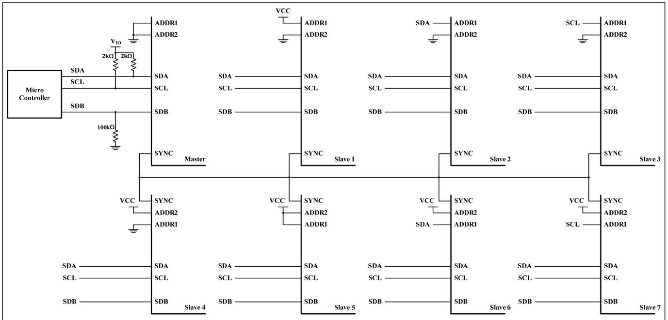
**Figure 2** Typical Application Circuit (Eight Parts Synchronization-Work)
