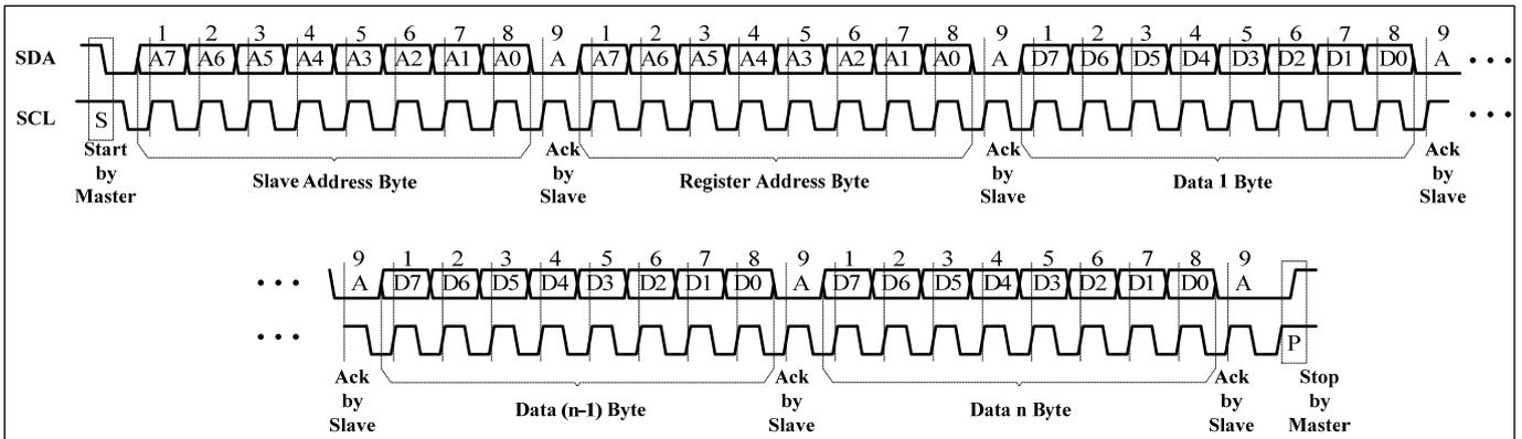
Figure 7 I2C Writing to IS31FL3745 (Automatic Address Increment)
