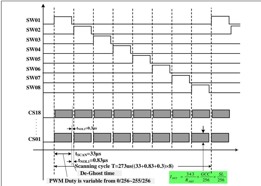
Figure 12 Scanning Timing
