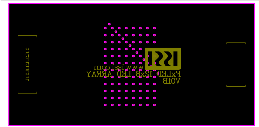
Figure 10: LED Board Component Placement Guide - Bottom Layer
