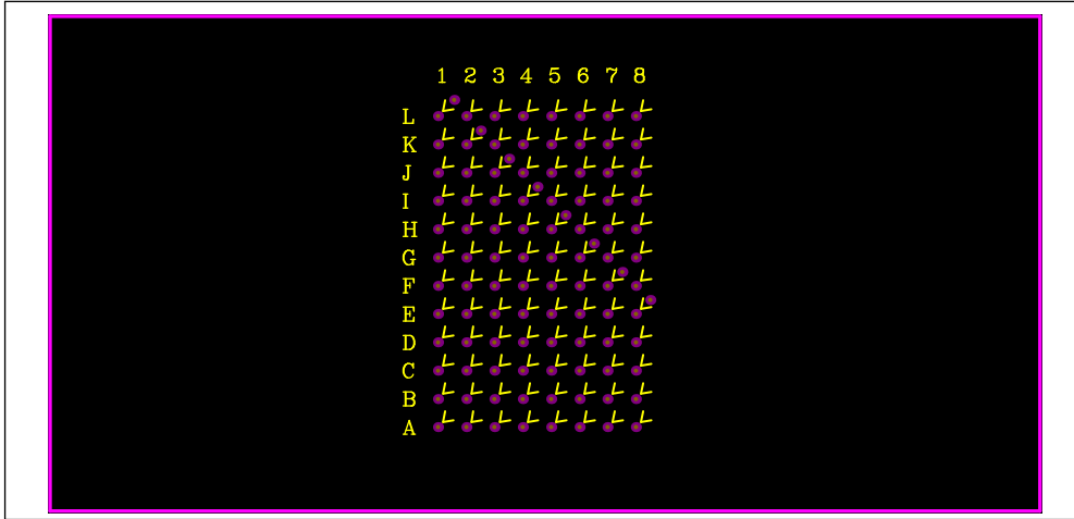
Figure 8: LED Board Component Placement Guide - Top Layer
