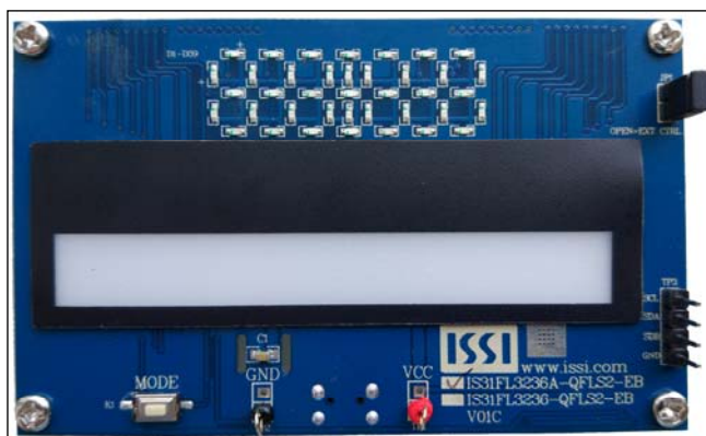
Figure 1: Photo of IS31FL3236A Evaluation Board
