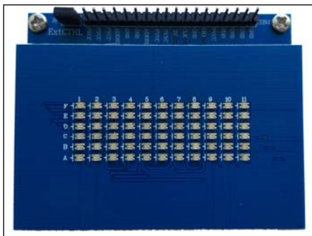
Figure 1: Photo of IS31FL3743B Evaluation Board
